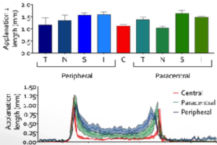
Fig. 11: Distribution of the applanation length. Top: Length at applanation 1 per position. Bottom: Applanation length over time, position grouped in zones.
