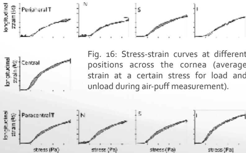
Fig. 16: Stress-strain curves at different positions across the cornea (average strain at a certain stress for load and unload during air-puff measurement).
